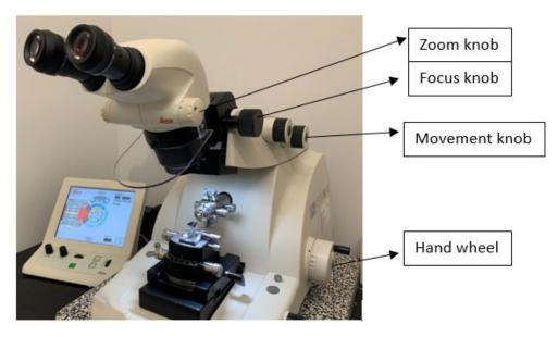
Use the hand wheel (on the right side) to bring the specimen to the same level as the knife edge.  Carefully move the knife forward until it is within about 1mm of the specimen block and lock the knife securely in place by the knife holder clamping screw.
