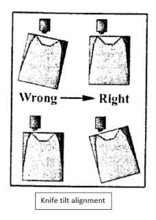
4) Tilt the sample block face up or down by the sample holder tilting screw to make the knife edge reflection on the top of the block face is equal to which on the bottom of the block face. After all the adjustments, the knife edge reflection is even side to side and stays the same width as the block is passed by the knife edge.
