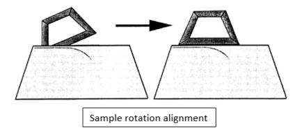
3) Rocking the sample up and down by the hand wheel to observe the knife edge reflection on the block face. Swing knife left or right by the knife swing screw to make the knife edge parallel to the block face (back off knife a little if needed before adjusting to avoid pump the sample block face).
