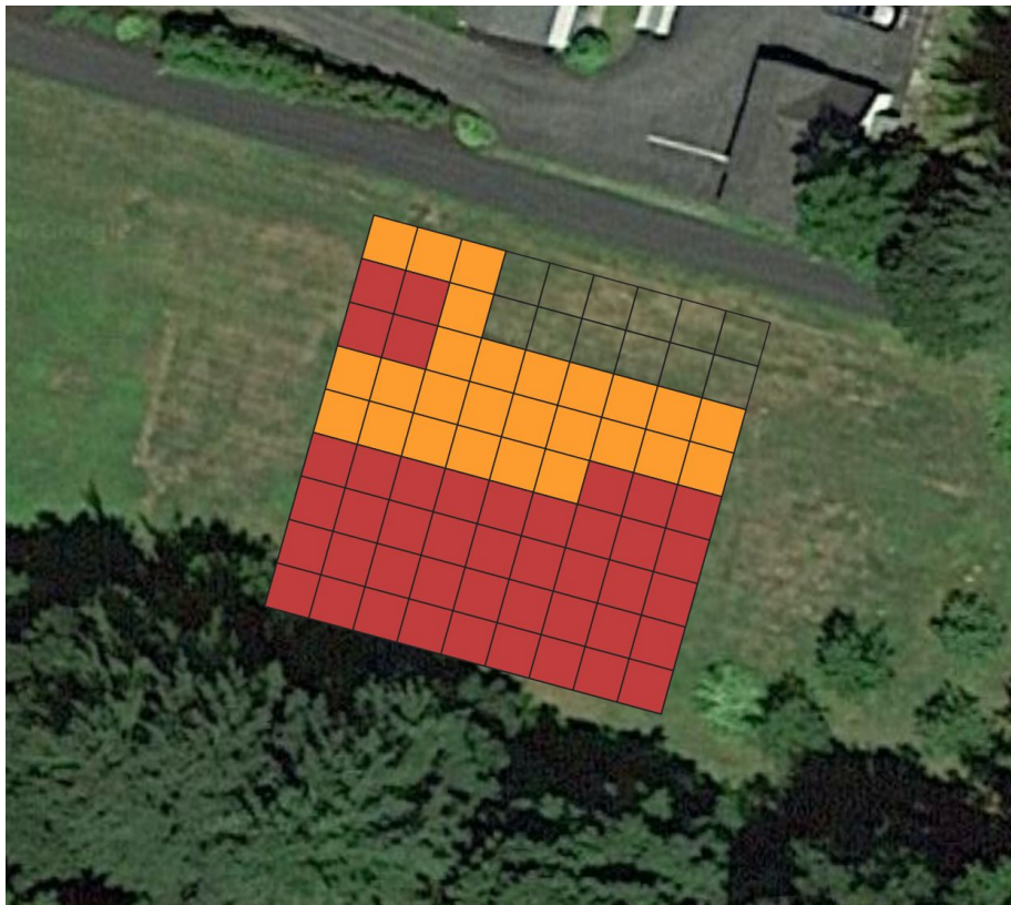
Figure 5. Cost analysis visualized. Red areas represent 17m 3 excavated, and red and orange areas combined represent 34.5m 3 excavated.
