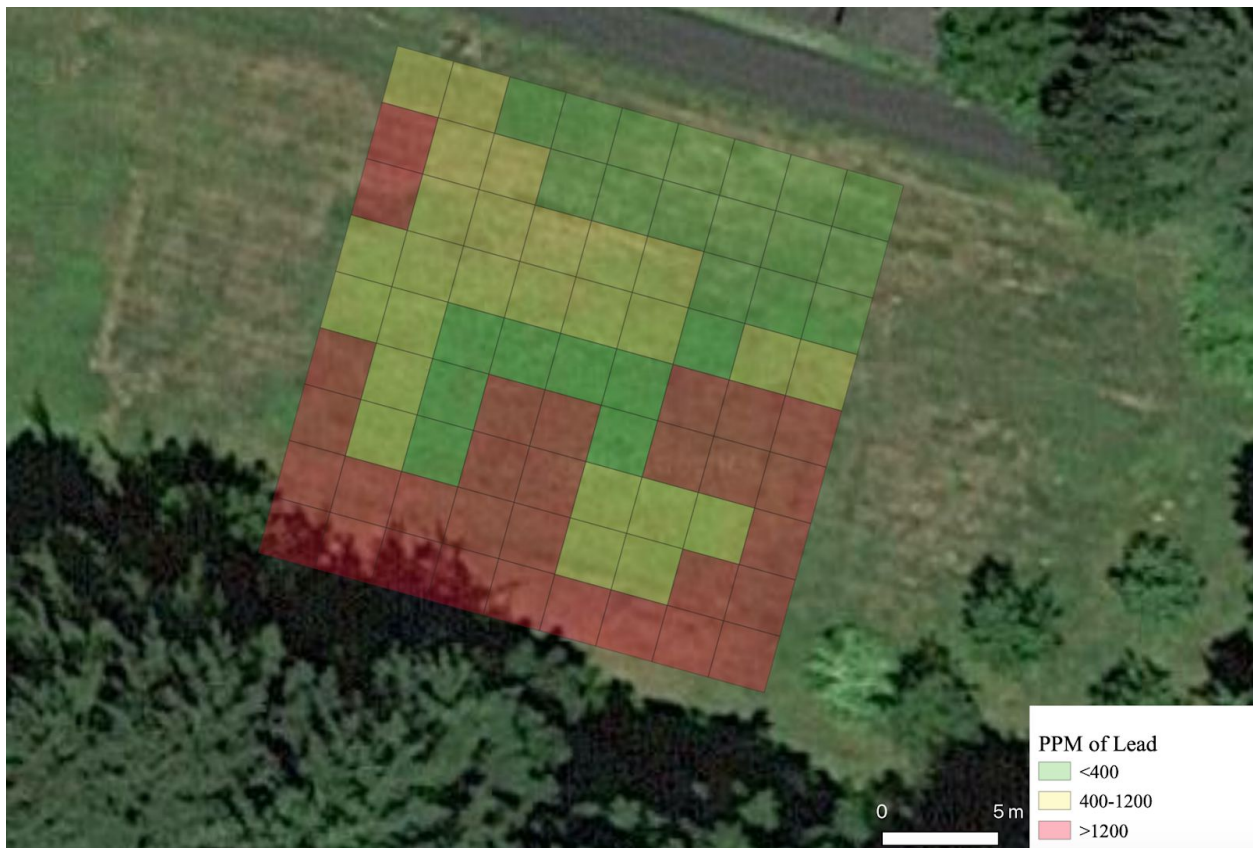
Figure 4. Lead concentrations categorized by EPA standards. Each cell (2.5m 2 ) represents the highest value at each of its corners and at both depths.
