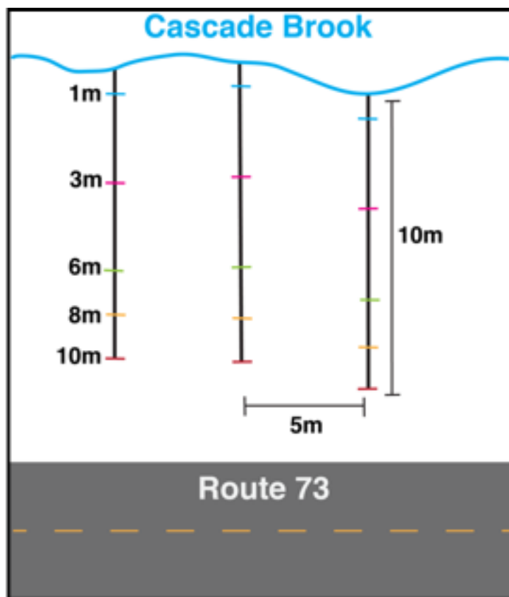
Figure 2: Example of transect methodology in relation to stream bank and route 73 at CB site (Not to scale).
