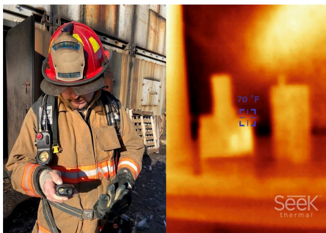
FIGURE 4.5. FIREFIGHTER USING THE SEEK THERMAL IMAGING CAMERA (LEFT) IMAGE FROM SEEK CAMERA OF C-AIR AND COMMERCIAL PARTICULATE MONITOR IN BURN FACILITY (RIGHT).
