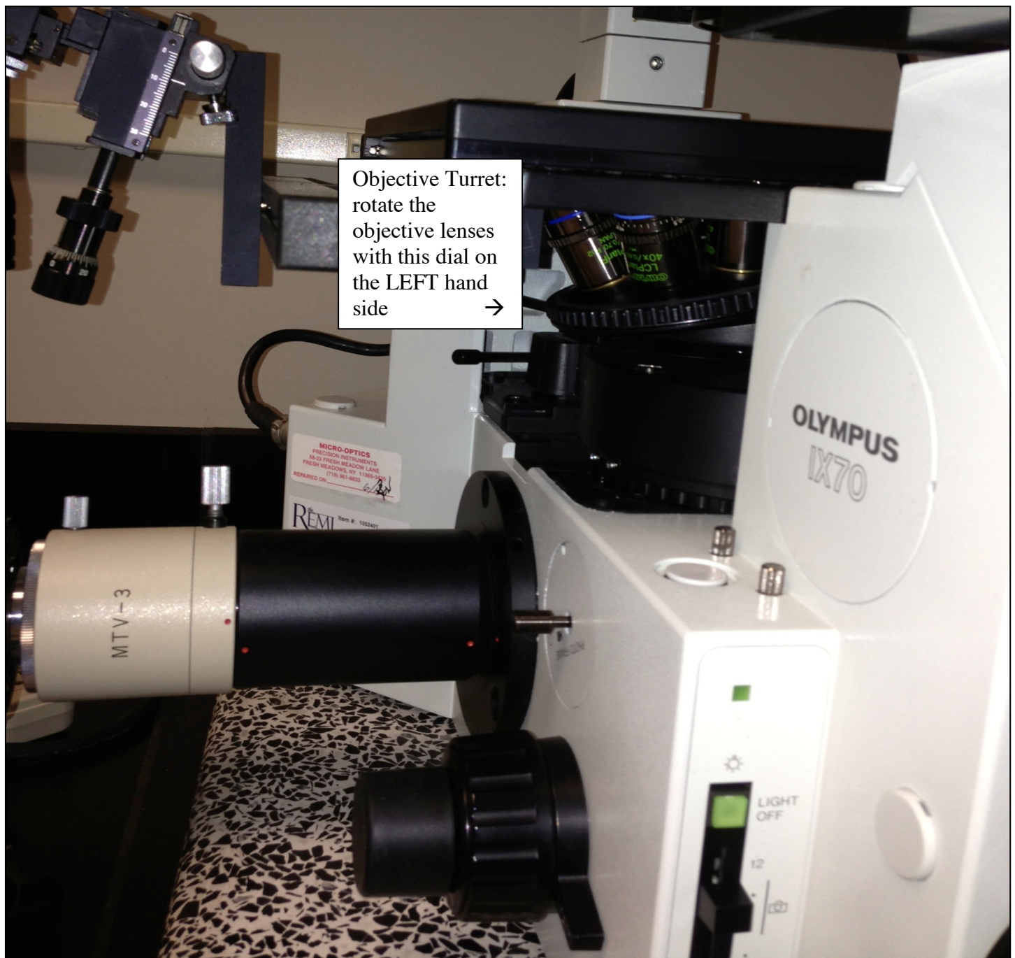
Fig. 1: Objective Turret. Be careful not to bump higher objectives into your specimen on the stage. Lower the objective turret (coarse focus knob) when going to higher objectives!
